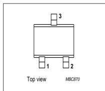
Fig.1 Simplified outline (SOT323) and pin configuration.
